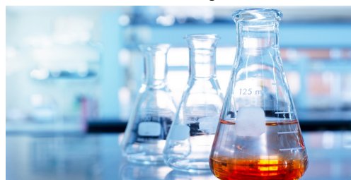
Figure 2: Erlenmeyer flasks, commonly used to mix, heat, and store liquids in laboratory experiments.
