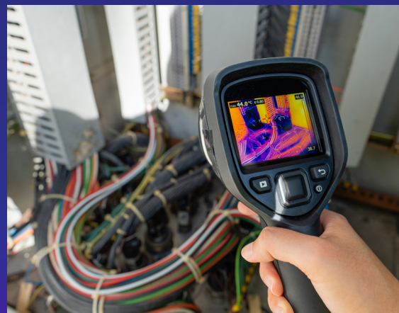
Figure 4: A thermal camera converts heat energy into a visible image
