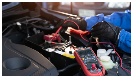
Figure 1: A technician measuring voltage of a car battery.
