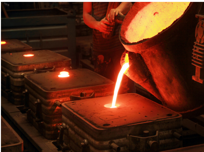
Figure 1: Molten metal being casted into a sand mold.
