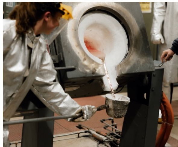
Figure 2: A METAL bootcamp participant obtaining molten metal from a furnace to pour into a mold.
