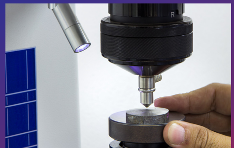
Figure 3: A hardness tester measures a material's resistance to dents, scratches, and wear.
