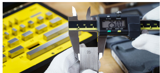
Figure 1: Calipers are used to measure objects with high precision.
